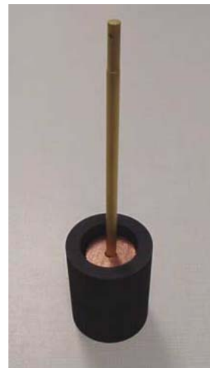
Figure 2 CVD TiN/TiC/TiCN/TiN Coated \alpha -SiC rod inserted in machined Cu placed inside graphite crucible.
