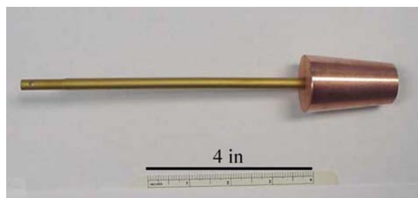
Figure 1 TiN/TiC/TiCN/TiN coated \alpha -SiC rod inserted in machined high purity, low oxygen Cu.
